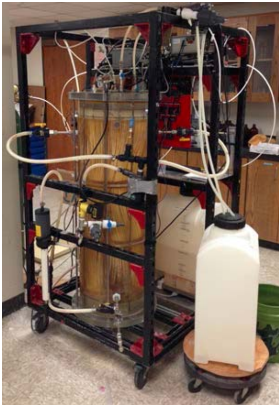
Counter-diffusion Membrane Aerated Nitrifying Denitrifying Reactor (CoMANDER) at Texas Tech University
