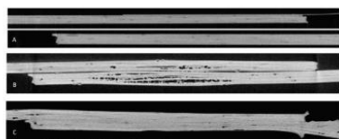
(A) Panels as fabricated, prior to welding (B) Panels after 1st microwave weld cycle, prior to lap shear testing (C) After lap shear testing, panels show improved bonding after 2nd microwave weld cycle
