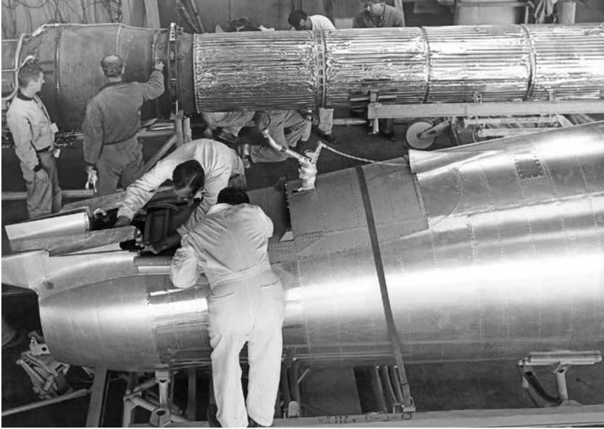
Two workers prepare to attach the vertical tail, foreground, while others inspect the engine and tailpipe assembly. (Laughlin Heritage Foundation)
