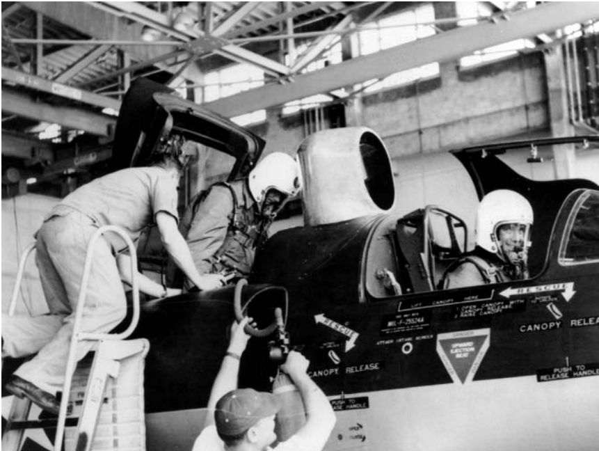
A second crew station had to be built to accommodate the sensor operator. (Lockheed Martin)
