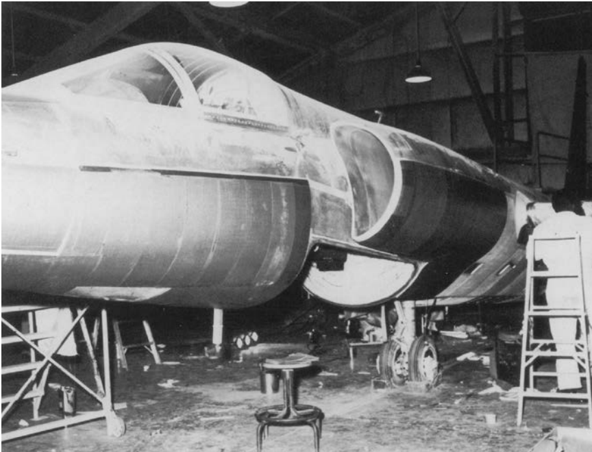
Engineers attempted two very different approaches to reducing the airplane's radar signature. One involved stringing ferrite beads on wires along the fuselage and wings while the other required coating parts of the aircraft with radar-absorbent material. (CIA)
