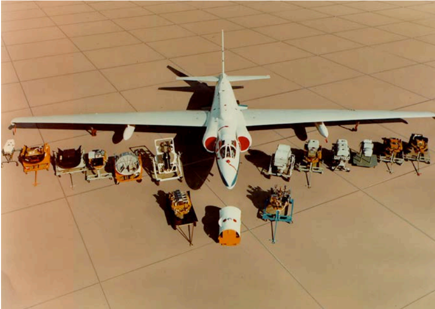
The U-2C was capable of carrying a variety of research instruments and cameras. (NASA)
