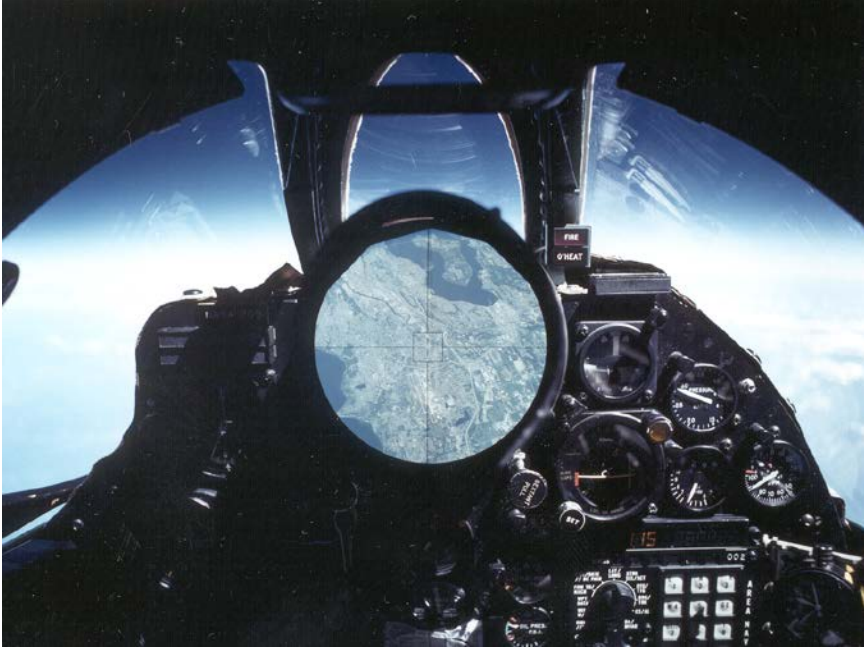
U-2 pilots found the driftsight, a downward-looking periscope, extremely useful for navigation. (NASA)
