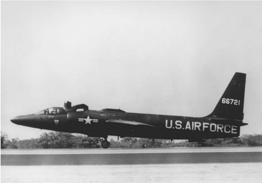
The final configuration of what came to be known as the U-2D. Note the cylindrical sensor housing between the canopies. (Lockheed Martin)
