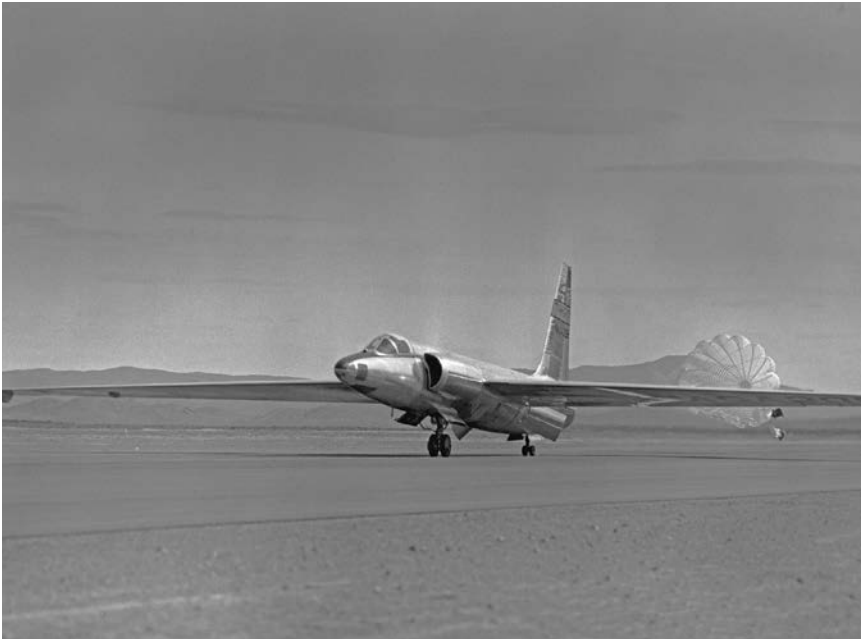
A U-2A is slowed by a drag chute during landing. (Laughlin Historical Foundation)
