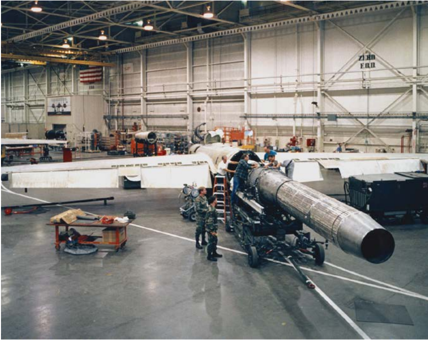
Technicians install a GE F118 engine in a U-2. (Lockheed Martin)
