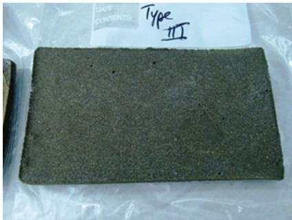
Figure 2. Foamed Basalt Test Samples for Analysis and Testing
