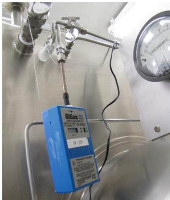
Figure 63: Gilian sampling pump and adsorbent tube for collecting organics in air.
