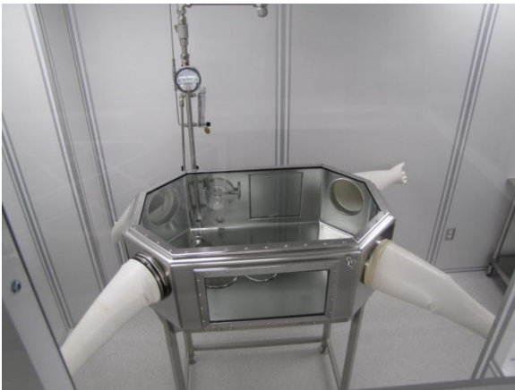
Figure 27: ACG inside the ISO class 5 cleanroom.
