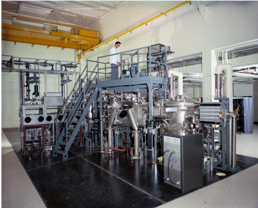
Figure 1: High Vacuum Complex during construction of the Lunar Receiving Laboratory in 1968 (NASA Photo # S68-25212).
