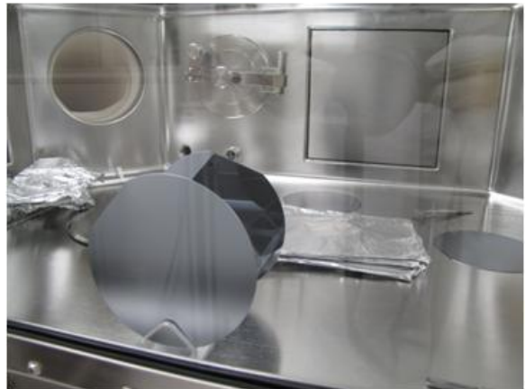
Figure 53: 6" silicon wafer vertical exposure in the ACG.
