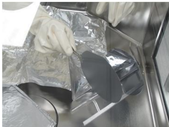
Figure 54: Silicon wafer handling during the ACG organic testing.
