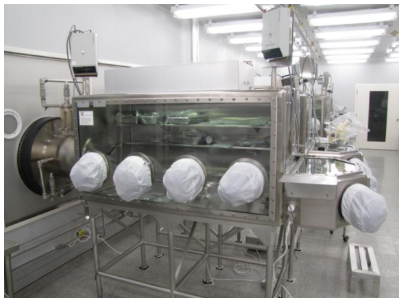
Figure 9: Lunar Lab Glovebox Apollo 16 – Cabinet 307-38 (PSL-38).
