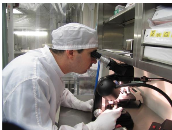
Figure 33: Stereomicroscope particle inspection of filter paper from UPW rinse.
