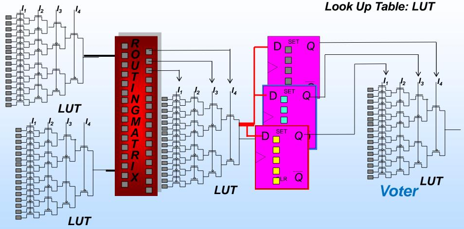
Too many other configuration bits + logic that can be corrupted by an SEU. Mitigation needs to be stronger than only protecting DFFs. To be presented by Melanie Berg at the NASA Electronic Parts and Packaging Program (NEPP) Electronics Technology Workshop (ETW), NASA Goddard
