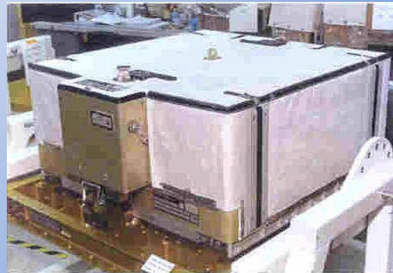
ISS Battery ORU Exterior
