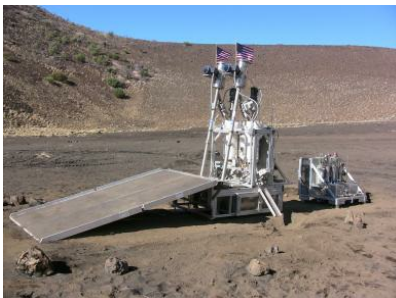
This is a hydrogen reduction ISRU plant for making oxygen from Regolith
