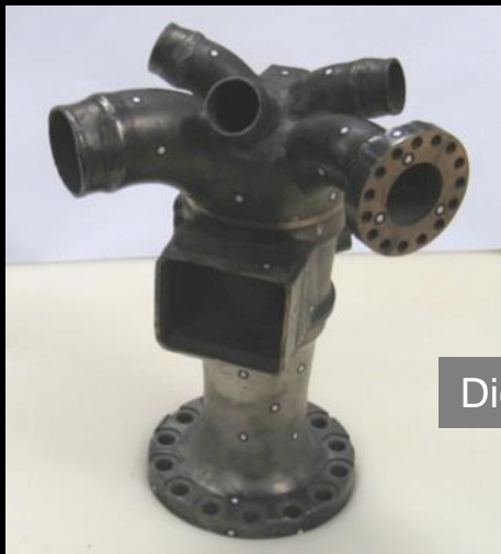
4. Series of simultaneous images and scans are processed in the software, and based on triangulation methods, the software will calculate 3D coordinates of the part and create a continuous contour
