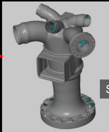
4. Series of simultaneous images and scans are processed in the software, and based on triangulation methods, the software will calculate 3D coordinates of the part and create a continuous contour
