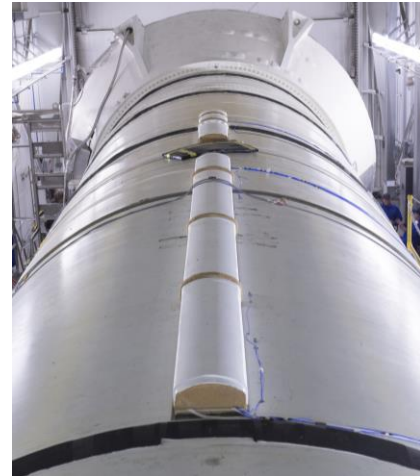
Figure 5. QM-1 systems tunnel simulator (black pad is process aid)
