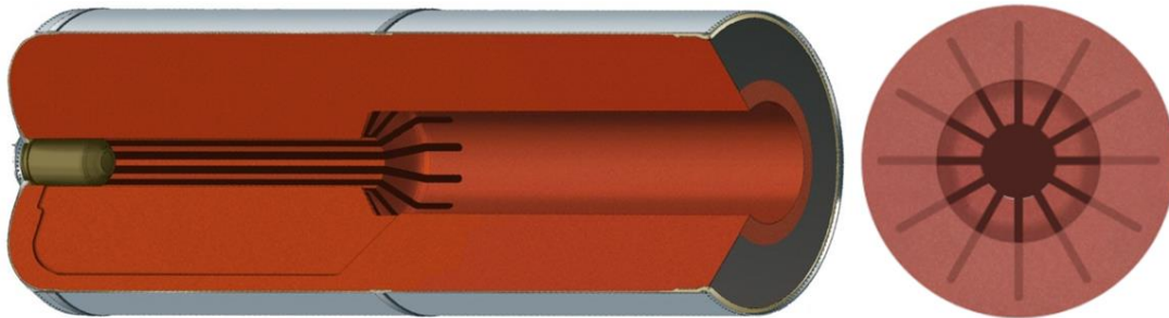
Figure 4. Forward segment grain geometry
