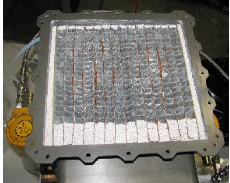
CDRA Sorbent Bed Cross Section
