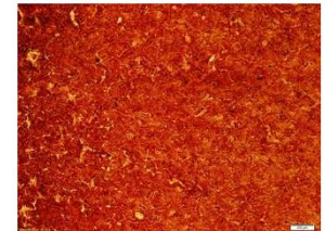
This optical microscope image of an etched copper sample helped scientists at NASA's Glenn Research Center in Cleveland, Ohio, as they characterized the quality of the copper for various build parameters for the copper liner. Credits: NASA/GRC/Ivan Locci
