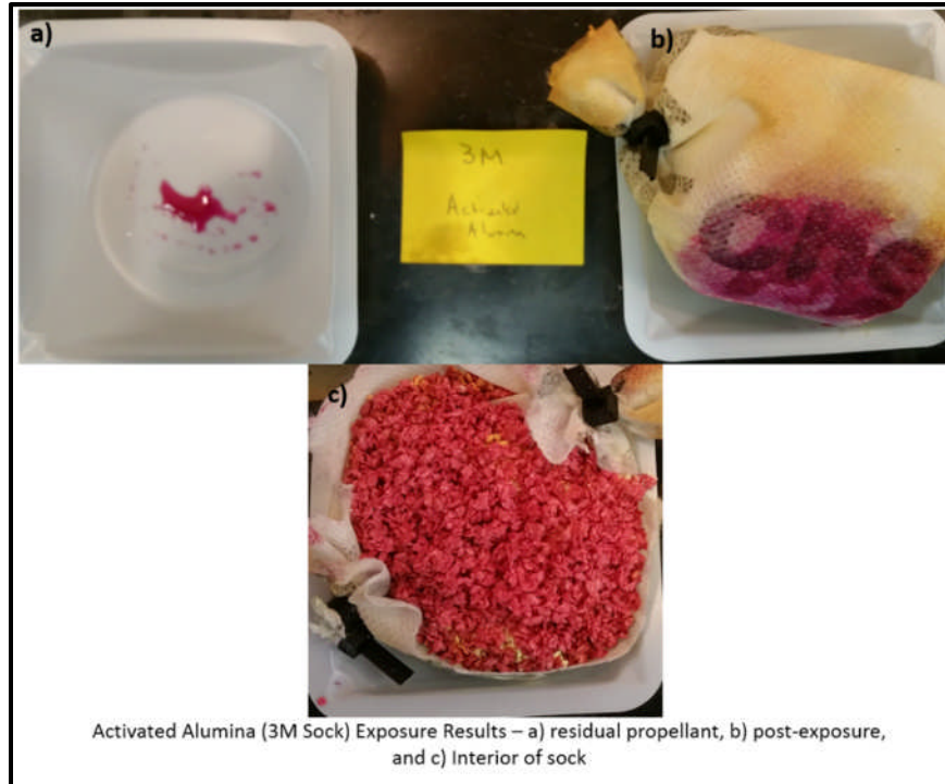
Figure 63. Activated Alumina (3M Sock) Exposure Results Showing Interior.
