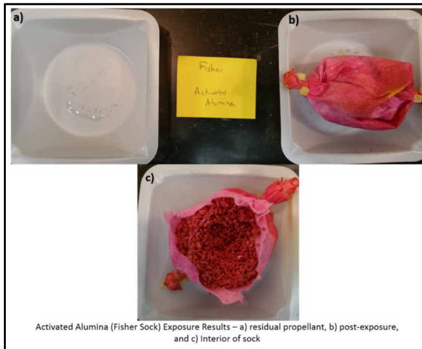
Figure 64. Activated Alumina (Fisher Sock) Exposure Results Showing Interior.
