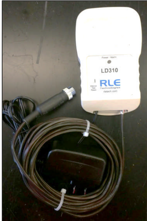
Figure 6. RLE Technologies SeaHawk LD310 Single Zone Monitor.
