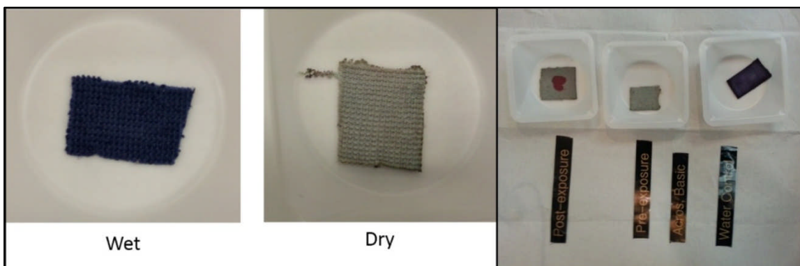
Figure 27. Acros Universal pH Indicator Solution (Basic) Indicator Wipes. Left – Wet and Vacuum Dried Wipes. Right – Exposure Results.
