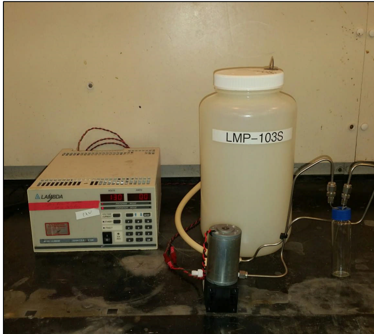
Figure 9. Setup for Evaluation of Active Sensors (LMP-103S).
