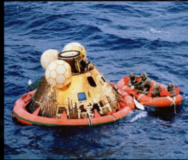
Inflatable airbags for Apollo water landing
