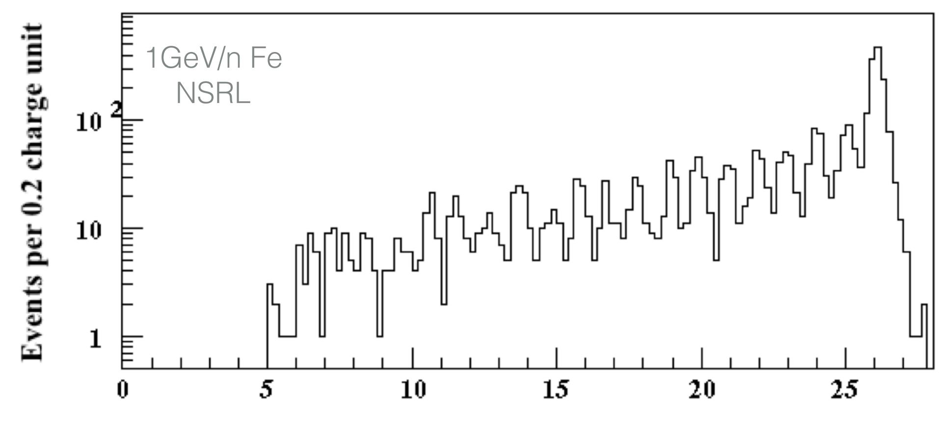
Intrinsic resolution of the system for monoenergetic ions can be seen to be well under 1 charge unit.
