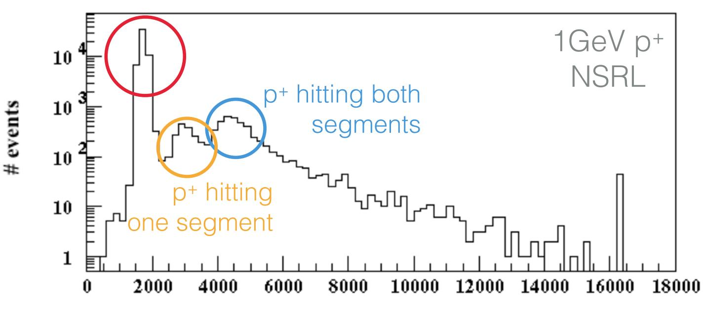
• C2 consists of two segments of the B diode wired together with one segment of the C diode (Si); calibration is straightforward, the relation between pulse height and deposited
