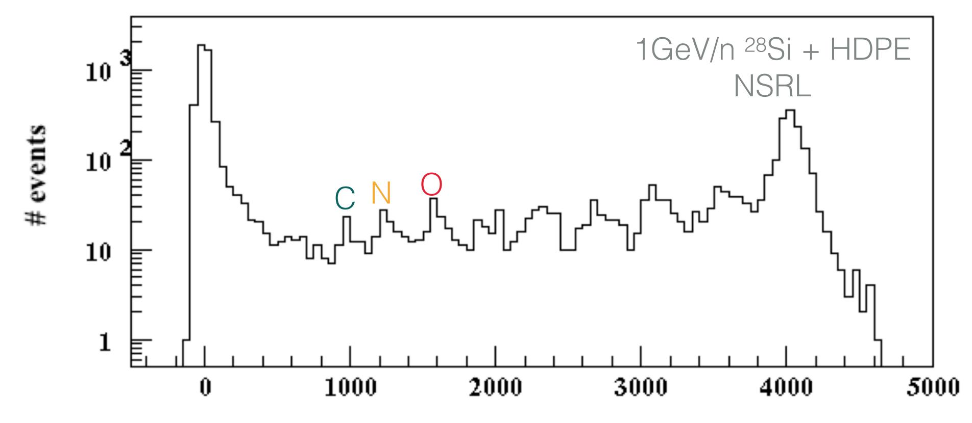
• Limited charge resolution in the space radiation environment; determined by the overlapping  $\Delta E$ distributions of different ions at different energies, but we are within the allotted 2e units.
