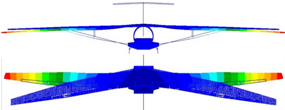
Figure 2.141 – Flutter Mode 2.70Hz, 1.09Vd Model, Residual Fuel, 356 KEAS
