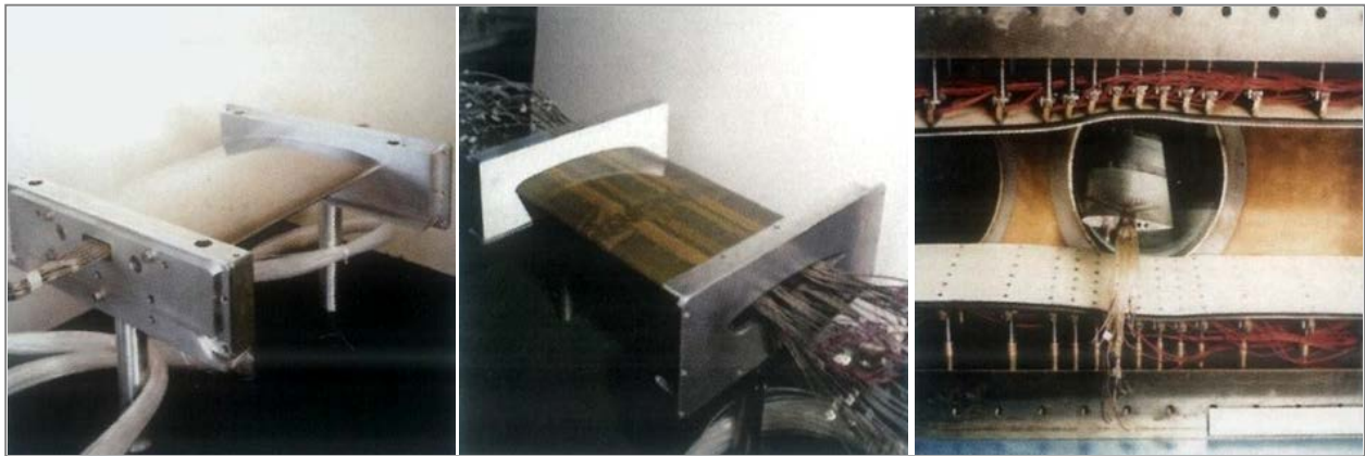
Figure 4.1 – Installation of 2D Airfoil Model in 0.3 meter Transonic Cryogenic Tunnel
