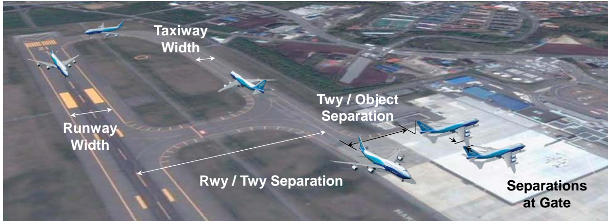
Figure 2.4 – Areas Impacted by Aircraft Wingspan
