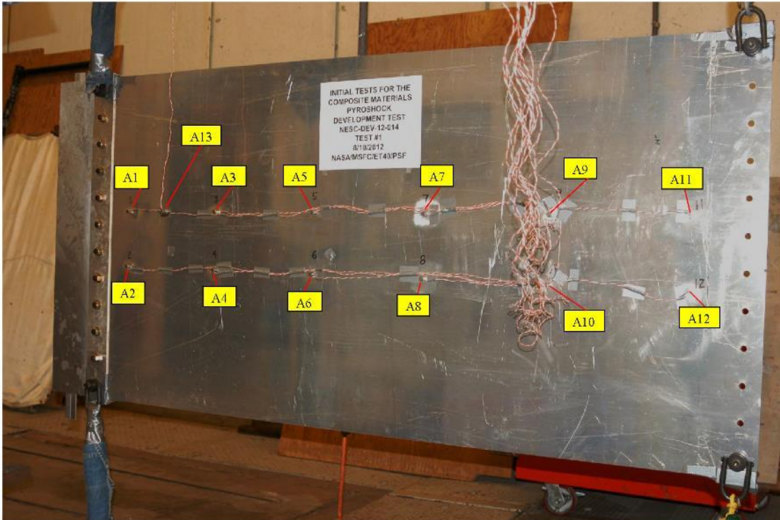
Accelerometer Locations, Test T01
