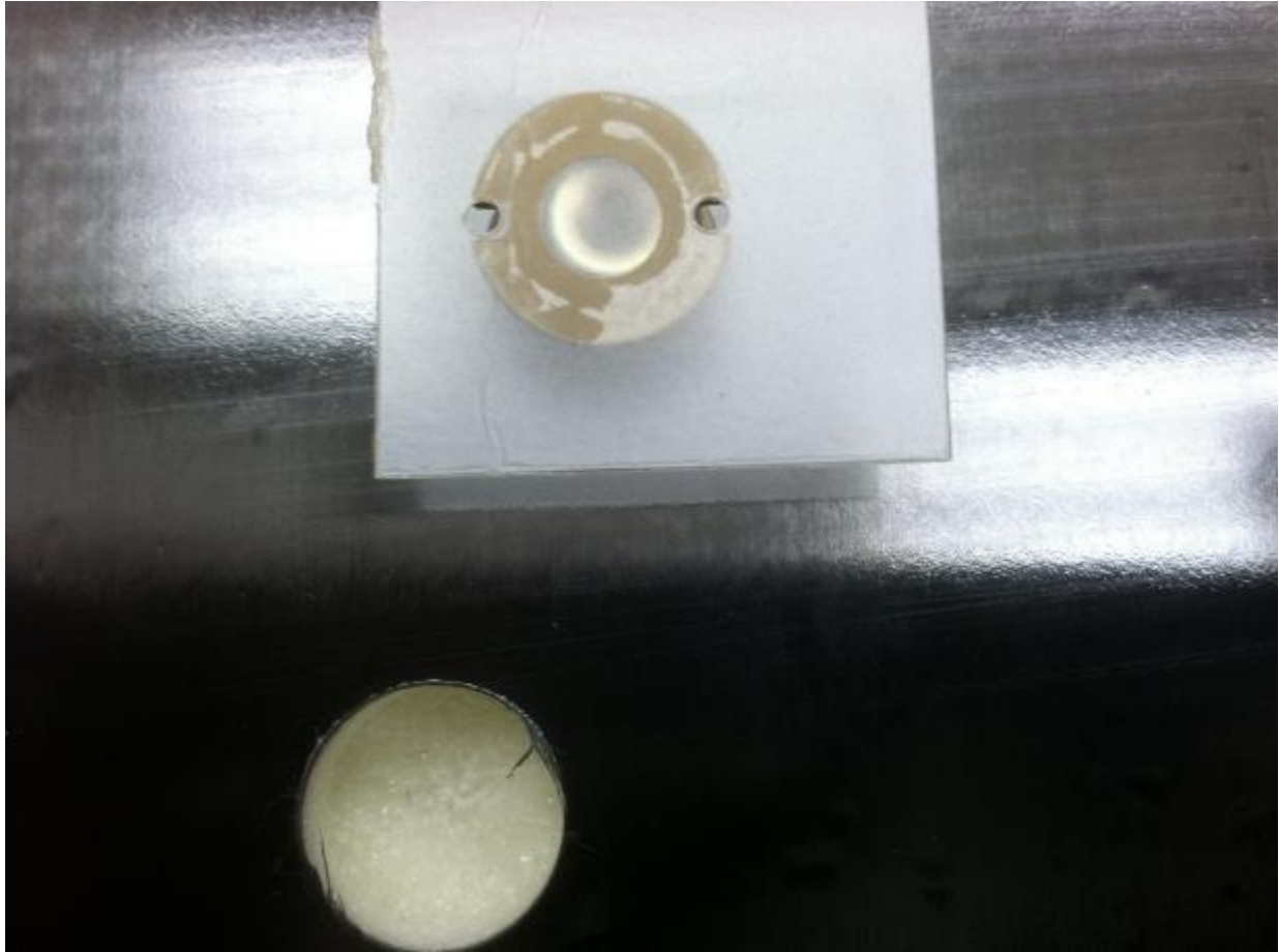
Figure A22. ROHACELL® Foam Sandwich Panel Prepped for Insert Installation
