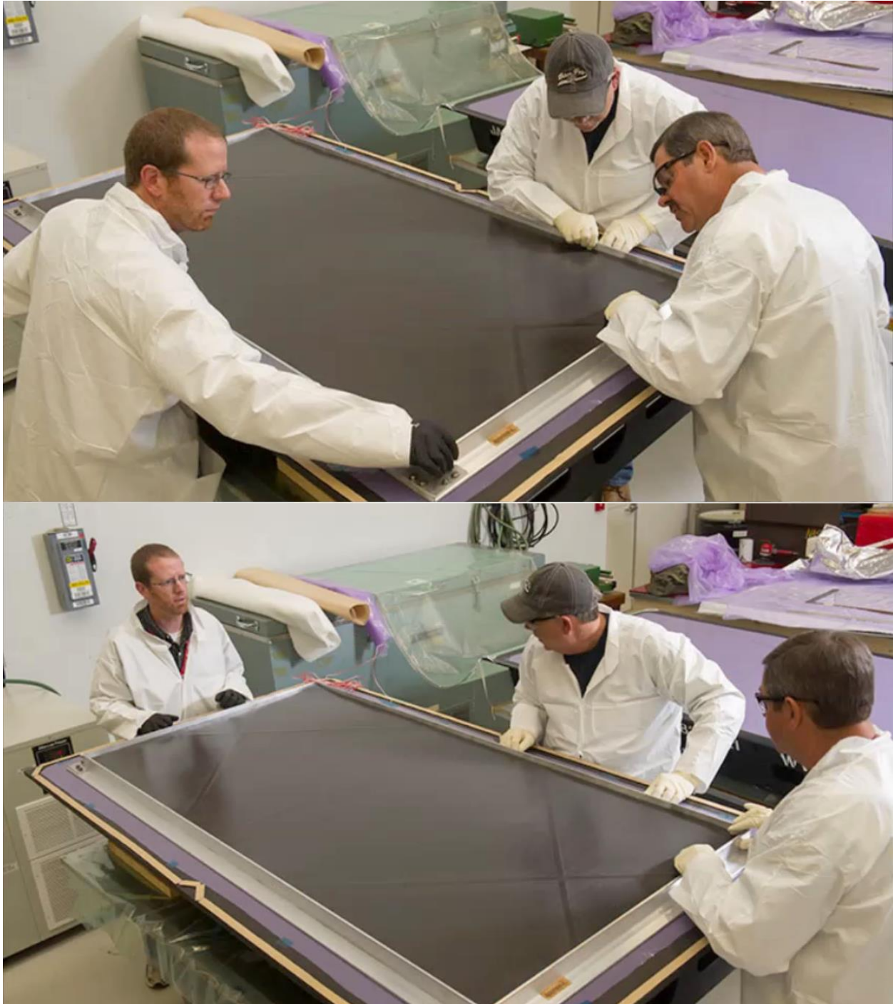
Figure A30. Composite Sandwich Panel Fabrication – Pictorial Presentation
