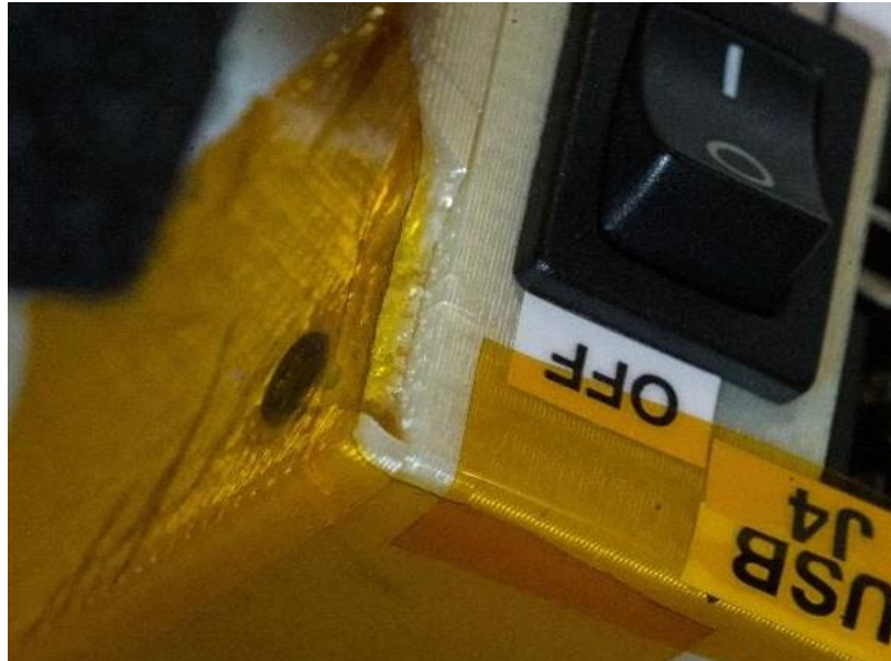
Figure 1: Image of the broken 3-D printed part onboard the ISS *Image property of NASA SPHERES
