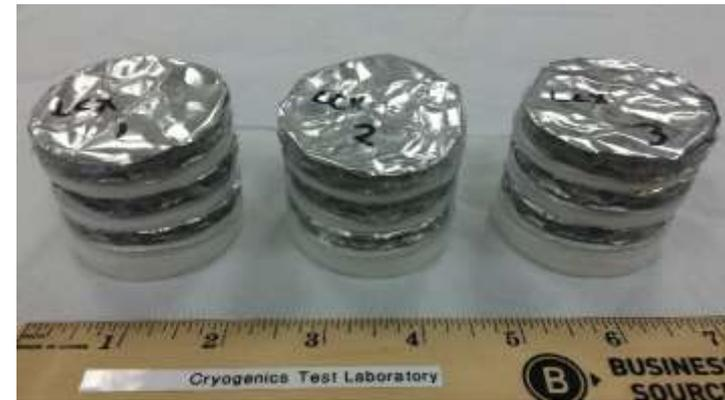
Exposure test specimens of LCX six-layer stack system.
