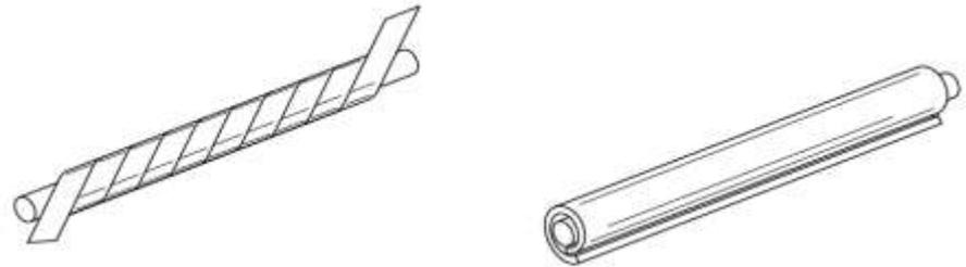
Small-diameter piping and tubing insulation wrap: spiral style (left) and cigar style (right).
