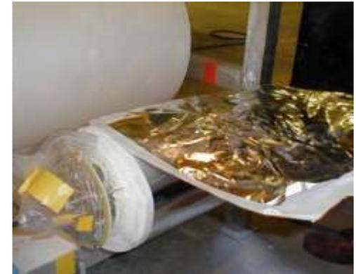
LCI production: The three components are layered by a continuous roll-wrap process.
