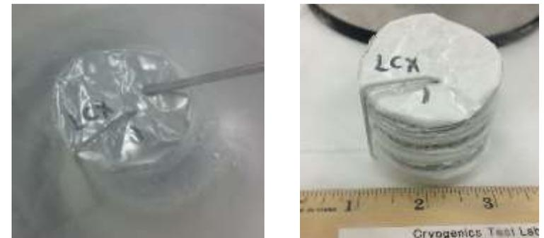
Extreme (cryo-water) exposure test: during LN<sub>2</sub> soak (left); after water bath (right).
