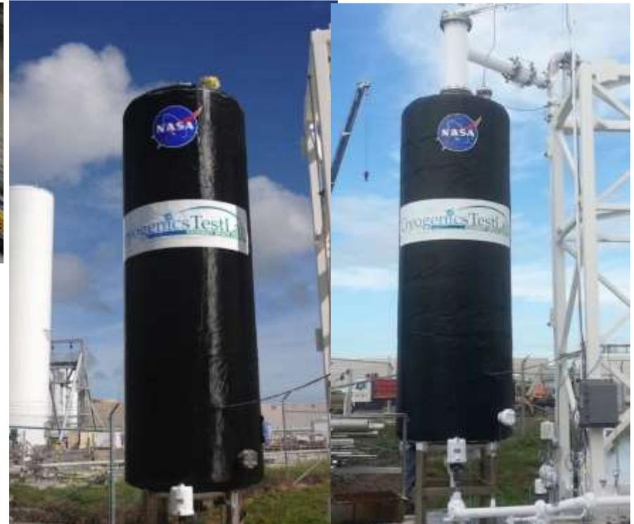
Vertical cylindrical cryogenic tank (7570-liter capacity) for flight tank simulation: completed LCX installation (left); during operation, fully loaded with LN<sub>2</sub> (right).
