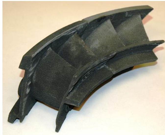
High pressure turbine nozzle segments: cooled doublet vane sections.
