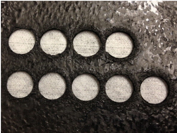
SEM specimens cut with different laser power/speeds
