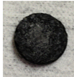
Laser cut prepregs used for composite processing
