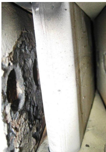
EBC Coated Prepreg SiC/SiC vane after 21 hour testing at 2500°F
