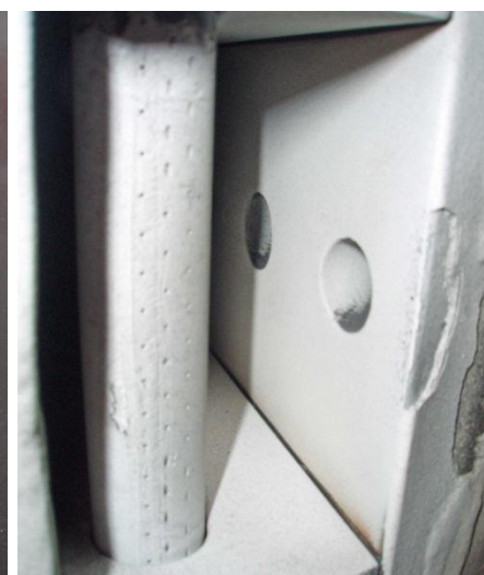
EBC Coated Prepreg SiC/SiC vane tested 75 hour testing at 2650°F
