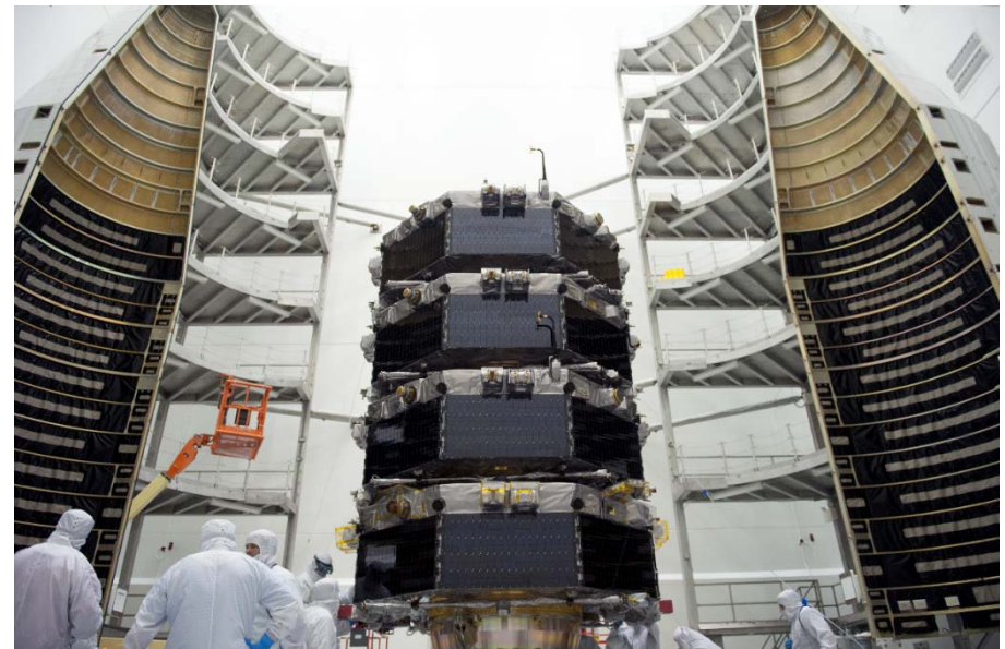
MMS Observatories being encapsulated in Atlas 4m Fairing
