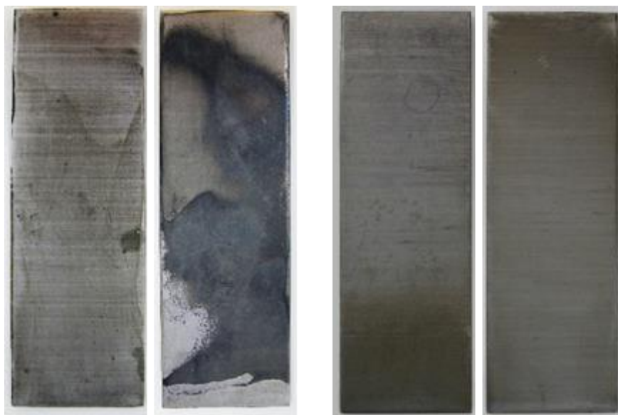
Figure 5: Front and back of Steel panels after immersion in 3.5% NaCl for 10 days Left: Front and back of Control; Right: Front and back of PPA inhibitor
