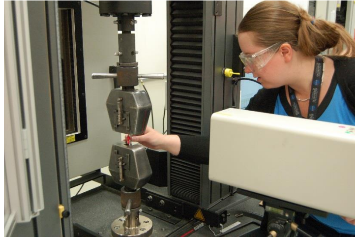
Figure 7. Sample Placement for Tensile Testing
