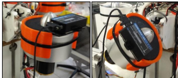
Figure 7: Microstrain IMU measuring thrust angle on Mini Free Flyer
