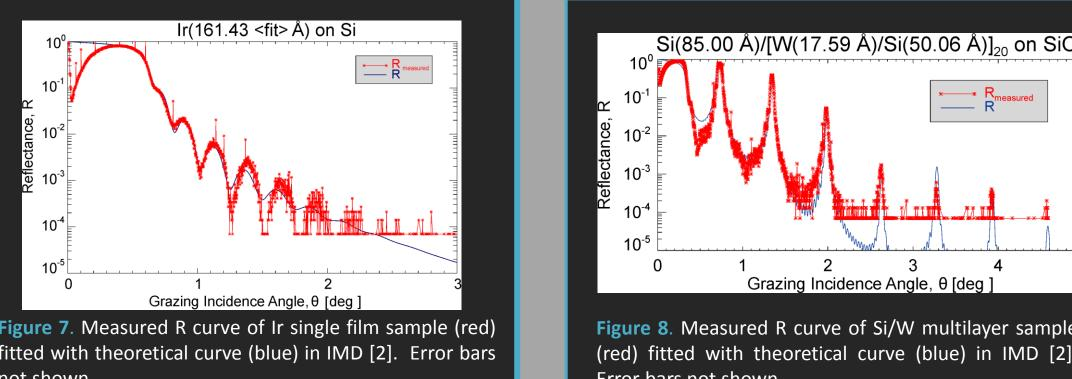
Figure 8. Measured R curve of Si/W multilayer sample (red) fitted with theoretical curve (blue) in IMD [2]. Error bars not shown.
