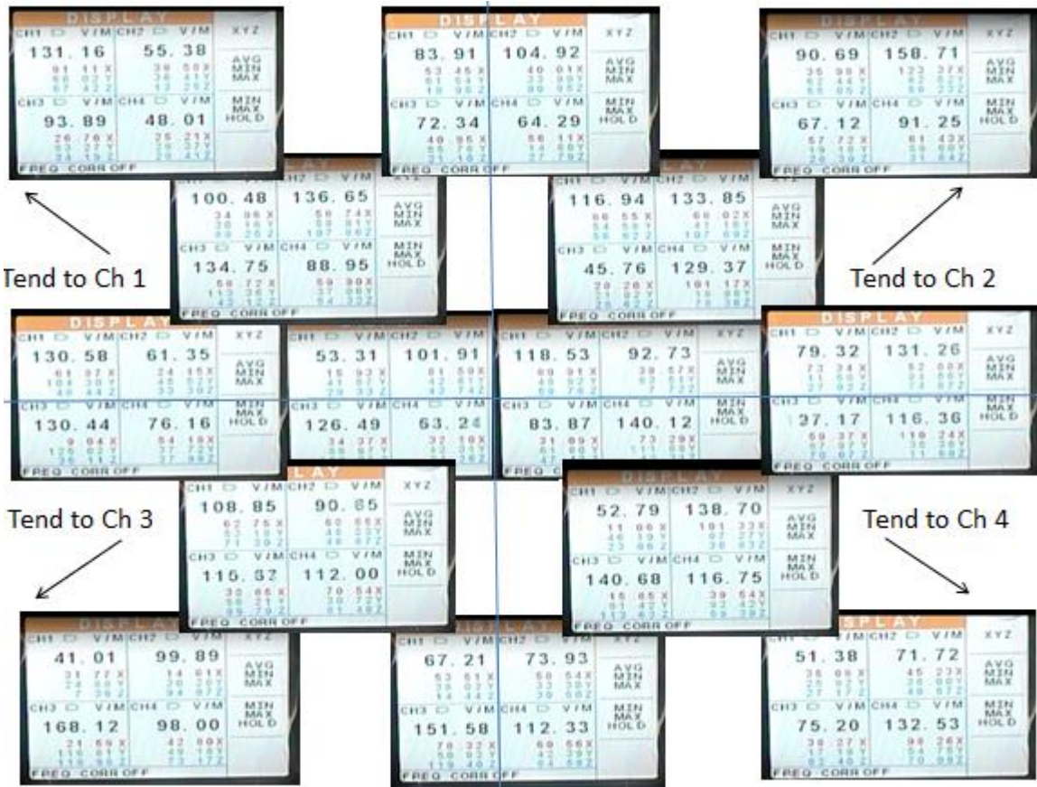
Figure 29: E-Field Probes Observed the RF Energy was “Stirring”
