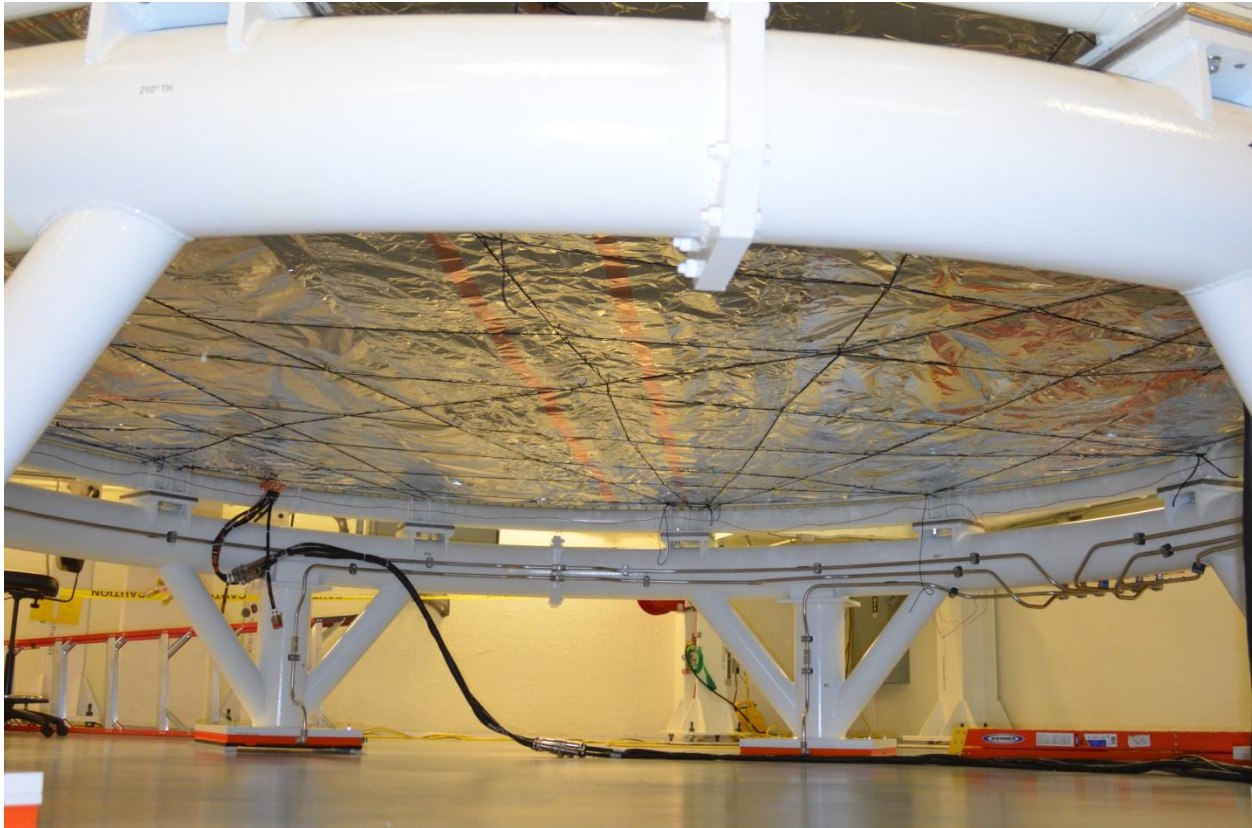
Figure 18: Service Module Bottom Closeout
