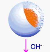
Microcontainer containing corrosion indicator, inhibitor or self healing agents
