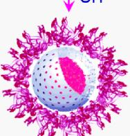
Contents are released from the microcontainer when corrosion occurs
