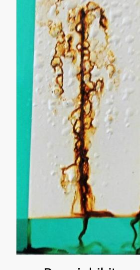
Carbon Steel; Waterborne Acrylic Coating; Salt Spray; 790 hours Inorganic particles
