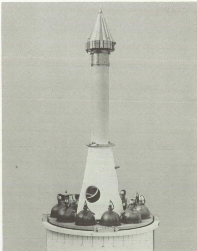
Fig. 1. Moon-Probe Vehicle Showing Pioneer IV Mounted on Titanium-Cased Fourth-Stage Rocket Motor
