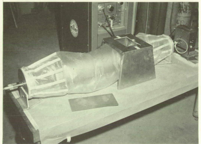
Fig. 7. Plastic Enclosure Used to Weld Titanium Motor Case
