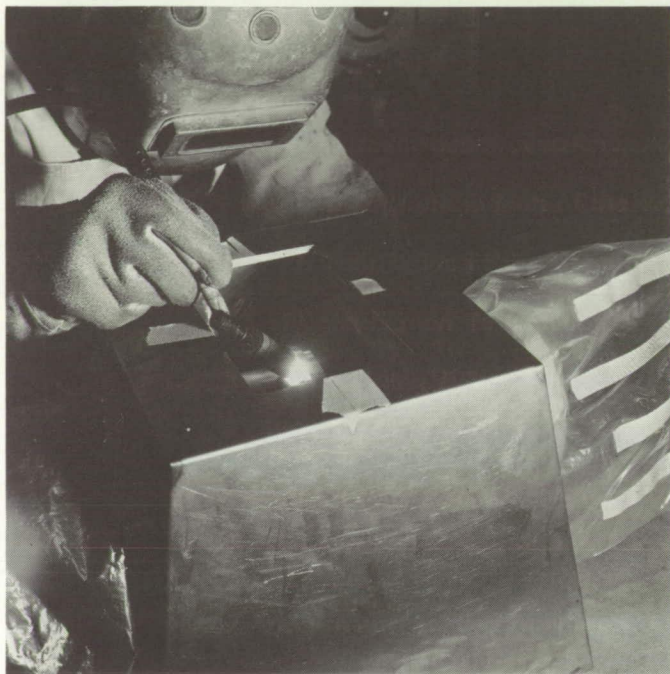
Fig. 9. Welding Alignment Ring to Shell
