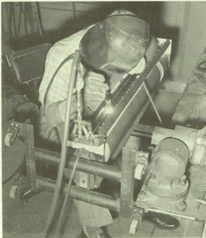
Fig. 6. Seam-Welding Titanium-Alloy Shell
