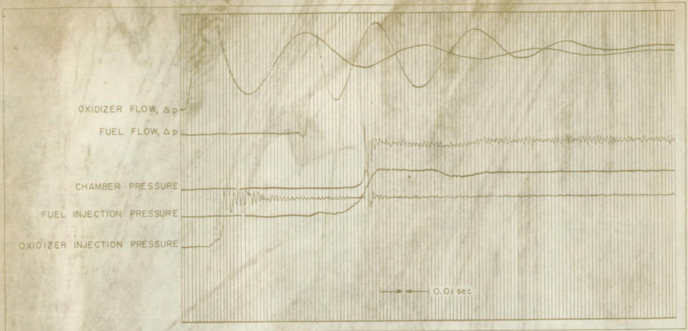
Fig. 23. Oscillograph Record of 800-lb-Thrust N_2O_4-N_2H_4 Motor Test with Injector Shown in Fig. 21
