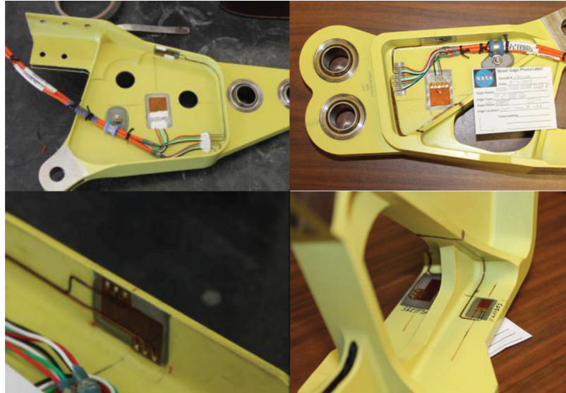
Figure 14. ACTE interface fitting strain gage installation.
