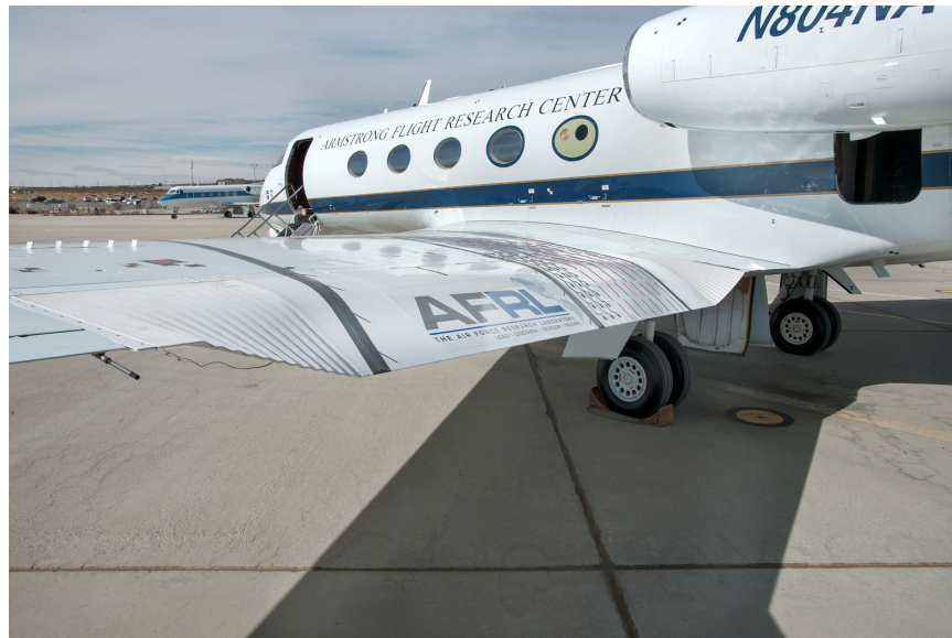
Figure 1. ACTE installed on the GIII at a flap deflection of 20^\circ .
