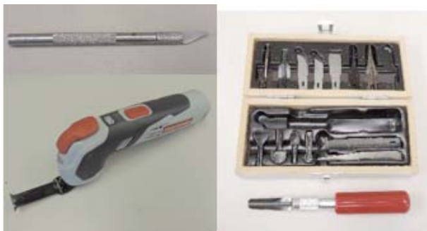
Fig. 20: X-acto knives and oscillating power tool used for extracting debris from high-density foam panels.
