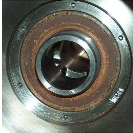
Figure 7. Corroded DA Centrifuge Bearing
