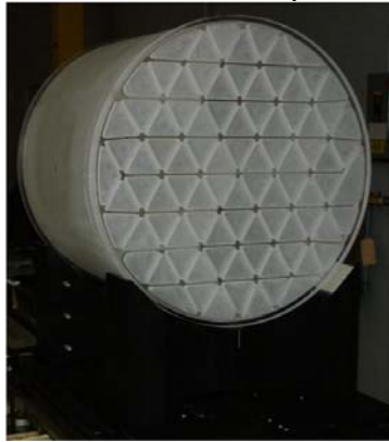
Figure 7 - A simple V-block mount was used to test the mirror horizontally during processing. This minimized the gravity effects during in-process testing
