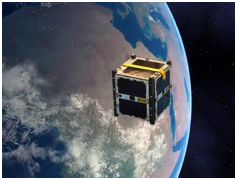
Figure 3: M-Cubed/COVE-2 is the reflight of a 1U CubeSat developed by U. Michigan to image the Earth carrying the JPL developed COVE technology validation experiment. Credits: NASA/JPL
