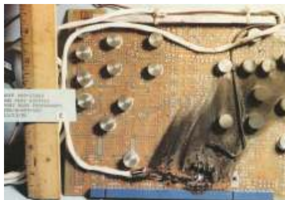
c. Posttest, minimal internal damage
