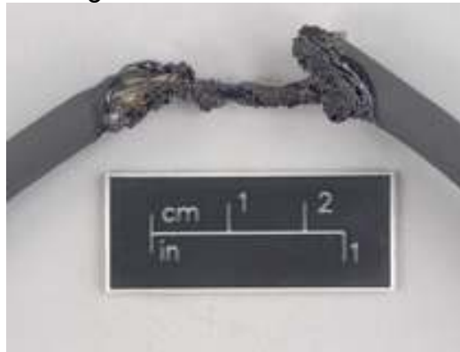
b. Damaged section of vacuum cleaner cable
