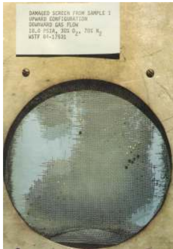
Figure 11. Damaged Aluminum Vent Screen from Airflow Tests
