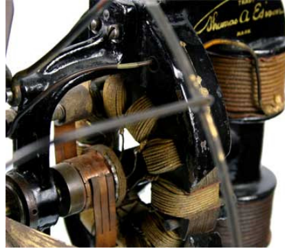
Figure 2.—Edison DC electric fan, courtesy of Spark Museum, Bellingham Washington.
