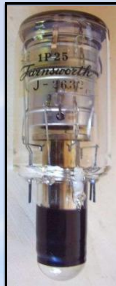
Original 1P25 image converter tube developed by RCA in the 1930's
