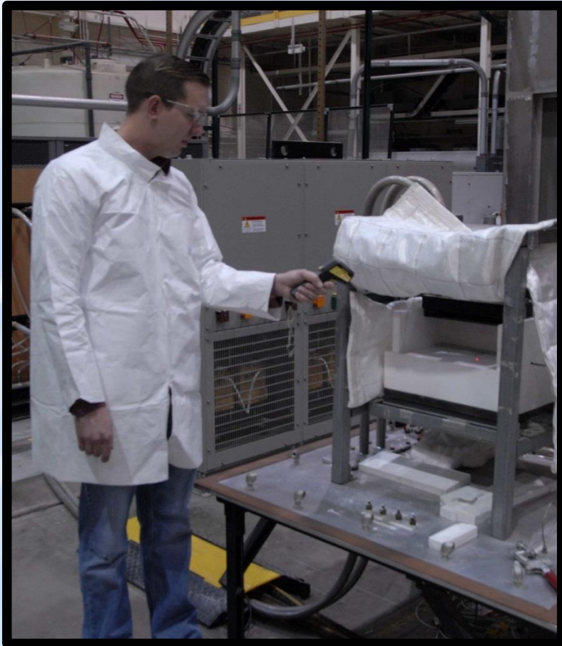
An engineer uses a readily available handheld radiation thermometer to measure the temperature of a furnace
