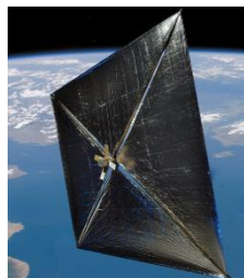
Figure 3. NanoSail-D solar sail. (Image credit: NASA Science News)
