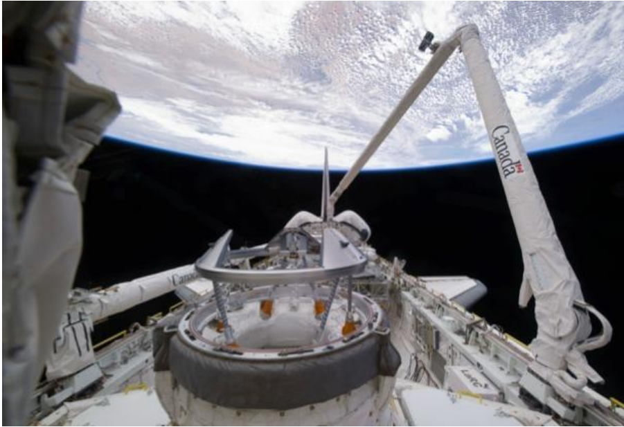
Figure 13. Shuttle Remote Manipulator System with Androgynous Peripheral Attach System (APAS) docking mechanism
