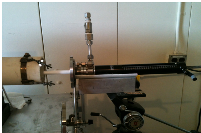
Figure 6.—New linear feed-through device for better control of doping process in the Stage 1 Furnace.
