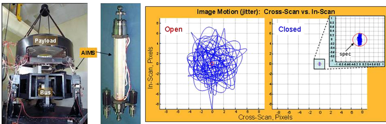
Fig. 7 Effectiveness of 2.5-m dynamic testbed for control of dynamic disturbances.
