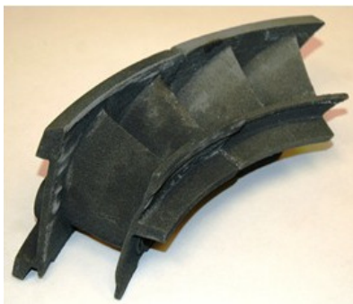
Figure 7: Demonstration of the additive manufacturing of turbine engine CMC components (20 vol. % SiC fiber). Two smaller first stage nozzle segments in addition to two high pressure turbine nozzle segments for a cooled doublet vane (top). Aligned cooled double vane sections (bottom).
