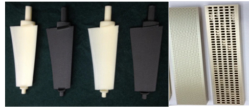
Figure 3: Inlet Guide Vanes (IGVs) and Acoustic liner fabricated using Fused Deposition Modeling (FDM).
