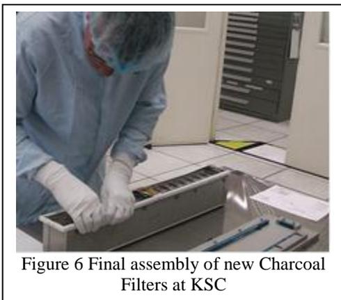
Figure 6 Final assembly of new Charcoal Filters at KSC
