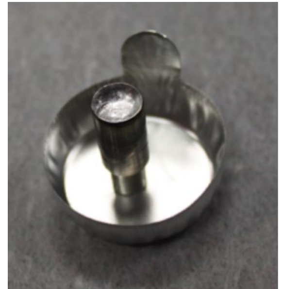
Quench vessel filled with a gallium-indium alloy
