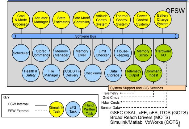
Figure 3. Layers of the Onboard Flight Software
