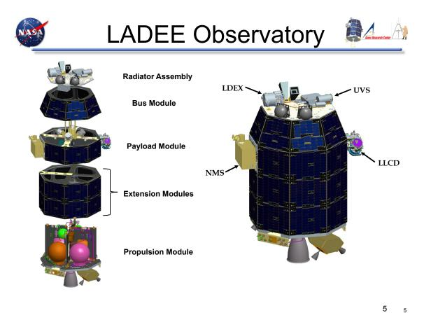
Figure 2. Picture of LADEE observatory, showing payloads and purpose of each assembly module.
