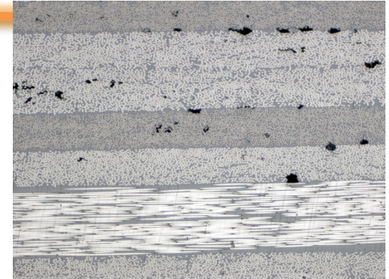
32-ply quasi isotropic panel, 100X
