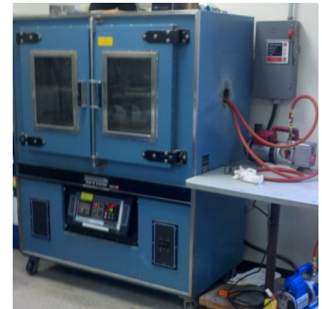
Oven Cure of Panel Under Vacuum
