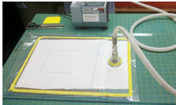
Vacuum Debulk of Composite Panel
