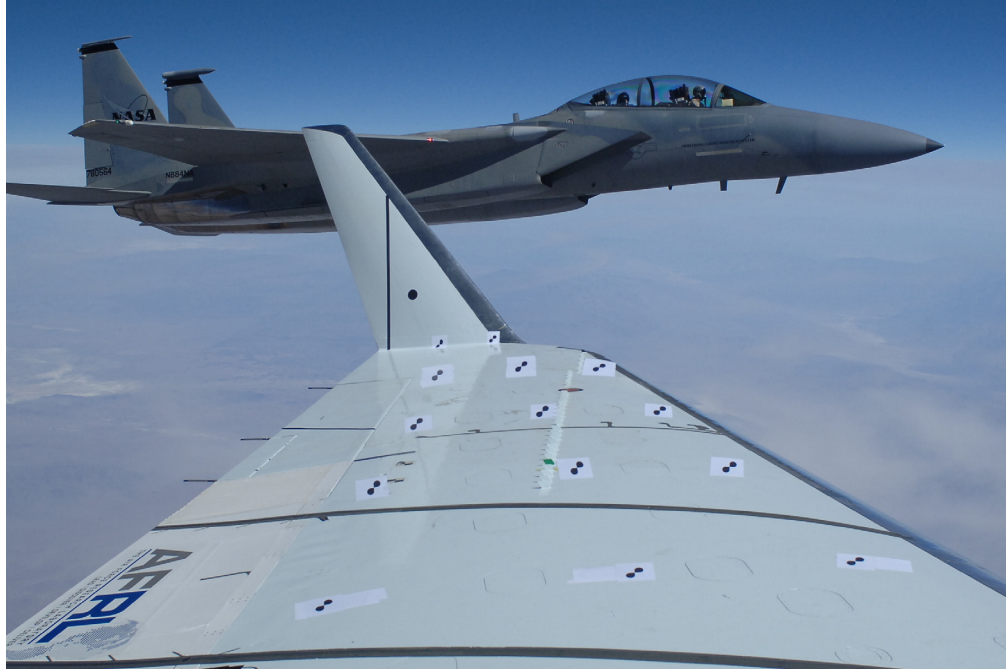
Figure 2. This photo of the Adaptive Compliant Trailing Edge (ACTE) was taken by an automated Wing Deflection Measurement System (WDMS) camera in the G-III that photographed the ACTE wing every second during the flight.
