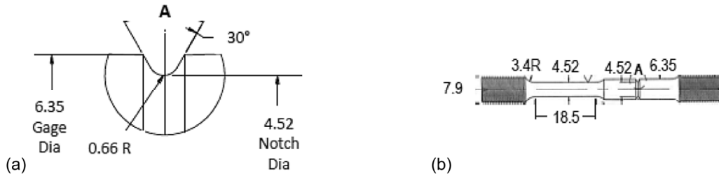
Figure 3.—Combo-bar specimen geometry. (a) Notch detail; (b) Specimen geometry.
