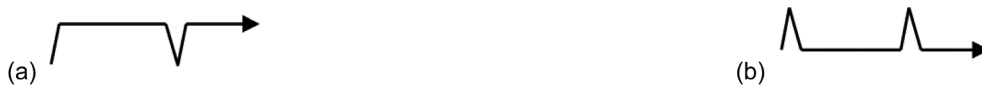
Figure 4.—The two dwell cycles utilized for the NLCF testing. (a) Max dwell: 1.5-90-1.5s. (b) Min dwell: 1.5-1.5-90s.
