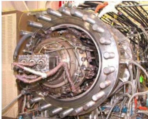
Advanced Subsonic Combustors (test rig at Glenn Research Center)
