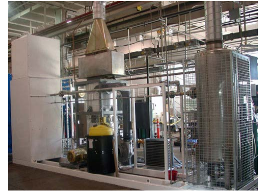
SCWO used for chemical weapon destruction (BlueGrass Army Depot 50 ton/day)
