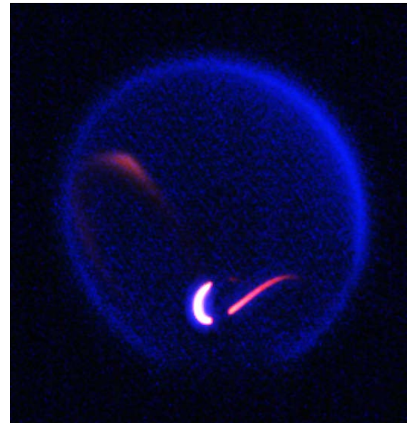
Spherical Non-Premixed Flame (formed with a porous sintered burner fed with gaseous fuel, where the image was brightened)
