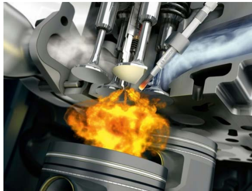
Diesel engine - high injection pressures
